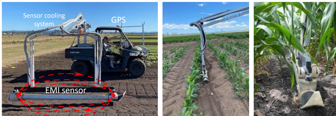
Figure 1. Example of the set up applied to the trial at Brookstead QLD, as described in Zhao et al., (2022).
