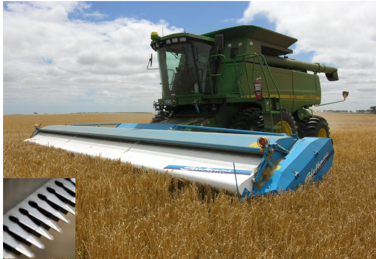
Figure 14. Stripper fronts use multiple rows of stripping fingers (inset) and help maximise the proportion of anchored residue retained in CA systems, e.g. Shelbourne Reynolds (picture by Glen Riethmuller)
