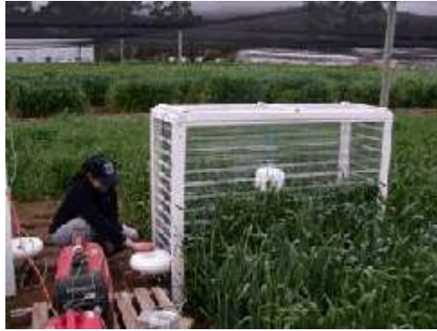
Image 1: Chamber set up in the field (left) over two rows of wheat, showing a heater at the bottom and TinyTag in a Stevenson screen hanging at canopy height within the chamber. Four chambers running at once (right).
