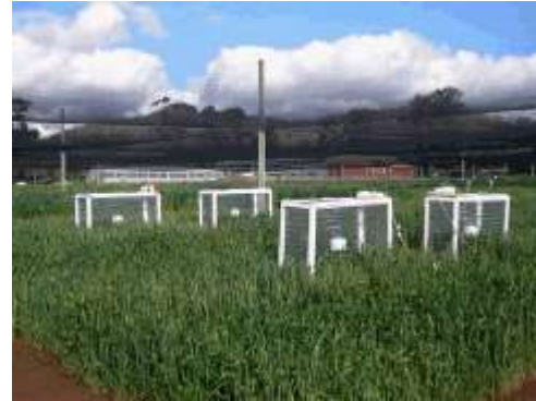
Image 1: Chamber set up in the field (left) over two rows of wheat, showing a heater at the bottom and TinyTag in a Stevenson screen hanging at canopy height within the chamber. Four chambers running at once (right).
