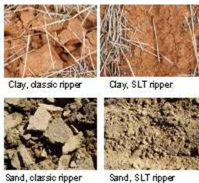
Figure 1. Clods resulting from ripping sandy and clayey soils with classic ripper and SLT ripper.
